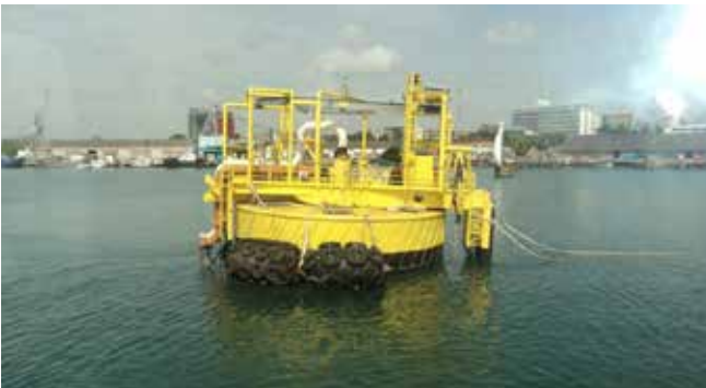
Single Point Mooring in Dar es Salaam
